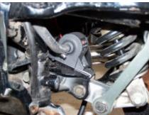
on front side first, by accessing over drive shaft), and then tighten both with Wrench. (Loctite is advisable as this clamp is not reachable after G
