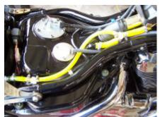
down). Cut 'stock tank' end of rubber vent hose approximately 3 ½" long. Insert new upside down 'Y' to this hose (slide stock vent hose further onto vent pipe to make room for 'Y').
