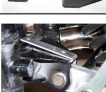
Place GTank under bike from left side (Remove lower left frame bar first, Bike should be on side stand during install).
